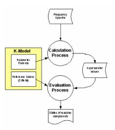
The first step in the analysis is to calculate frequency components related to faults defined by the Standard
